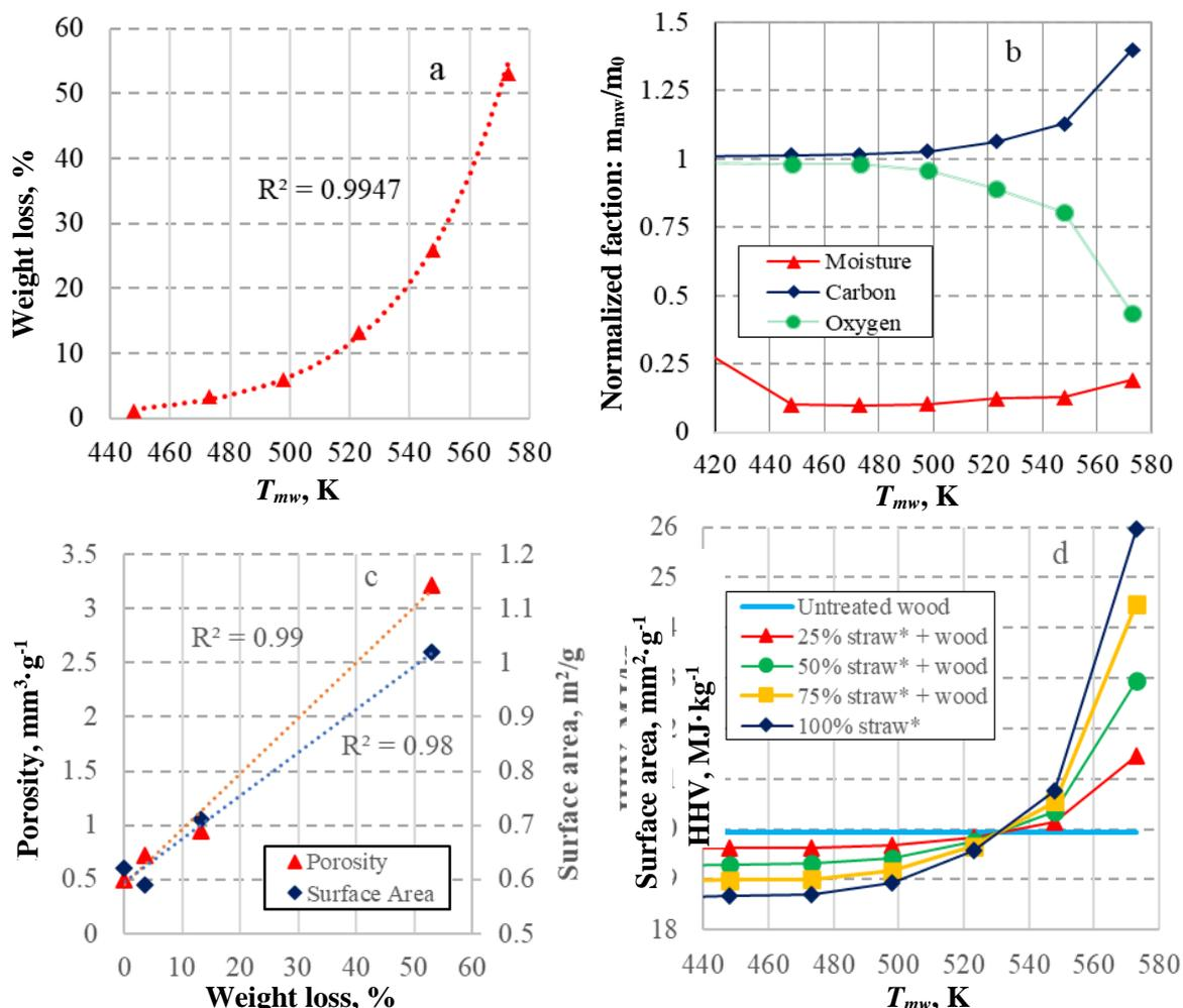
Fig. 1. Effect of wheat straw pellet pre-treatment on: a – weight loss; b – normalized elemental composition; c – porosity, surface area; d – HHV of blends with pre-treated straw and untreated wood as reference
