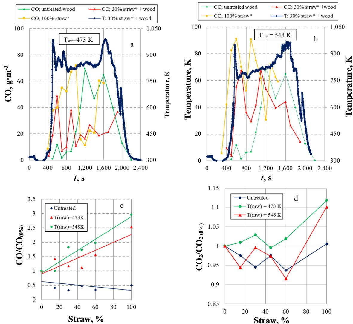
Fig. 3. Effect of variations of MW pre-treatment temperature and mass fraction of pre-treated wheat straw pellets in blends on: a – kinetics of the yield of volatiles  $T_{mw} = 473$  K; b – kinetics of the yield of volatiles  $T_{mw} = 548$  K; c, d – normalized average values of volatiles
